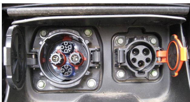
ZEO Leaf charging sockets: CHAdeMO (DC) left, Type 1 (AC) right.
